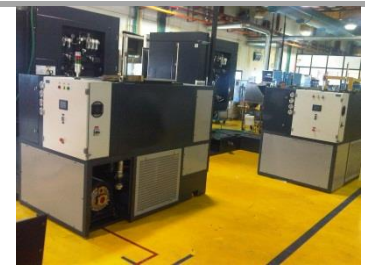
HP Combi Syst. with clean\dirty tanks on Makino G7 Aerospace grinder.
