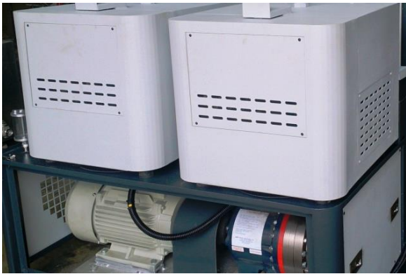
Aerospace Alloys Grinding System consisting of Centrifuge , Chiller, 70 Bar@30lpm and 40Bar@80lpm Hi Pressure pumps on " HAAS " Grinder
