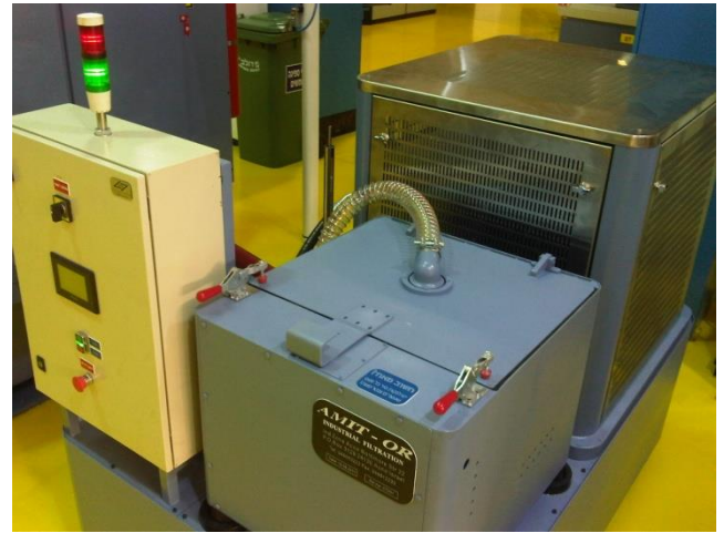
Carbide grinding system consisting of Centrifuge , Chiller, pumps for “ Anca “ Grinder
