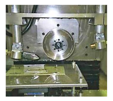
High Pressure cooling for grinding applications improves efficiency and reduces costs.
