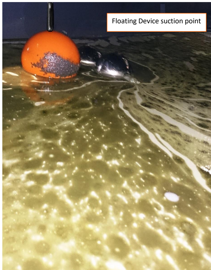
Floating device located inside Coolant Tank.
