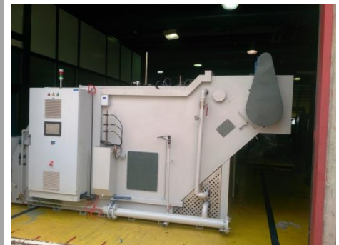
Vacuum Filter for Rough grinder Cincinnati on Emulsion
