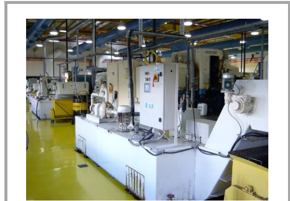
Mini Central units for 2 Excello grinders On SSU210 Viscous oil
