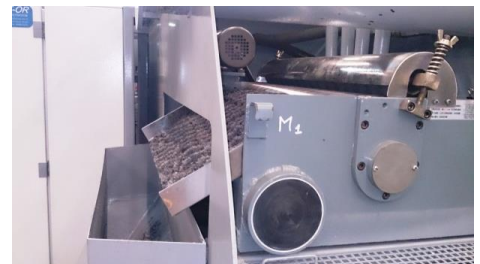
Vacuum Filter for Rough grinder Cincinnati on Emulsion
