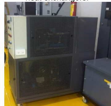
Net oil \ soluble SS 316 & machining at 20– 30 micron application suited with integral chiller.
